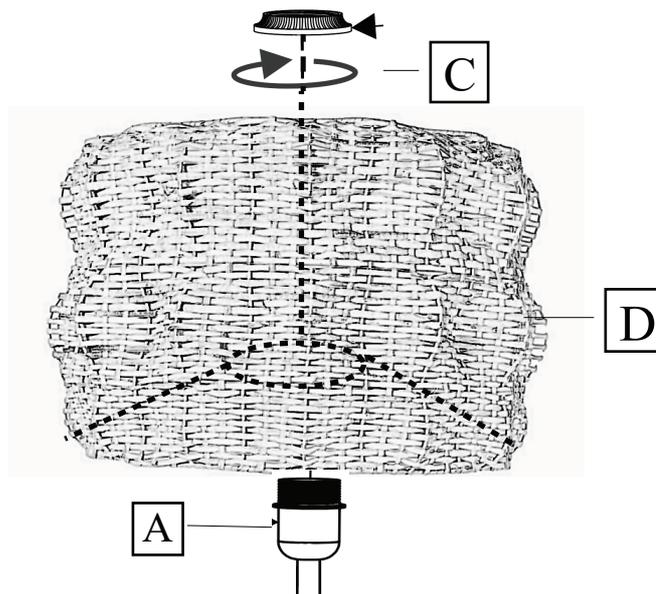
Remove Uno Ring (C) if it is pre-attached to light socket. Place Lamp Shade (D) onto the light socket on top of the assembly from Step 1. Secure by re-attaching Uno Ring (C) onto light socket. Tighten until snug. Remove any plastic wrapping on the Lamp Shade (D) before use.
