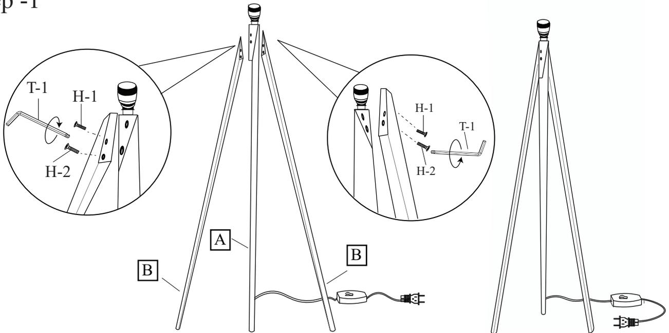
It is suggested to use a second person to assist you. Position Fixed Leg (A) and Detachable Base Legs (B) together as shown. Secure Detachable Base Legs (B) to Fixed Base Leg (A) with small Flat Head Allen Bolt (H-1) in the top holes, and large Flat Head Allen Bolt (H-2) in the bottom holes. Engage all bolts first, then fully tighten using the provided Allen Key (T-1). **DO NOT OVER TIGHTEN.**
