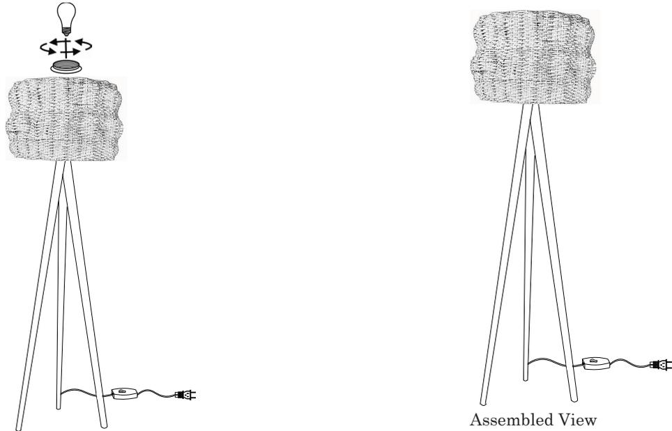
Insert Bulb (E; not included) into the light socket and rotate it clockwise to secure. Plug in lamp to a near socket and check for proper lighting operation. Assembly is not complete and the product is ready for use.
